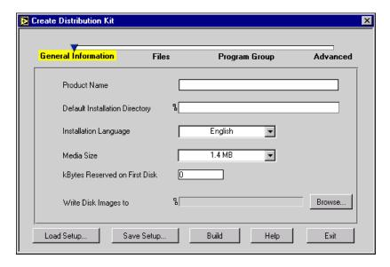
To create an installer, enter the information in this dialog box, then click the **Build** button at the bottom. This command compresses the files, builds an installer, and writes the disk images to the hard drive path specified in **Write Disk Images to**. You can run the installer image from that directory or copy it to floppies or other distribution media.
